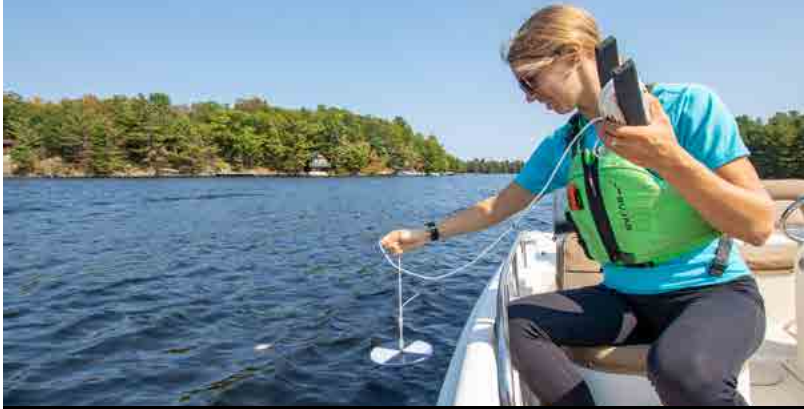
Lake Partner Program water clarity measurements are taken every two weeks throughout the summer using a Secchi disk.
