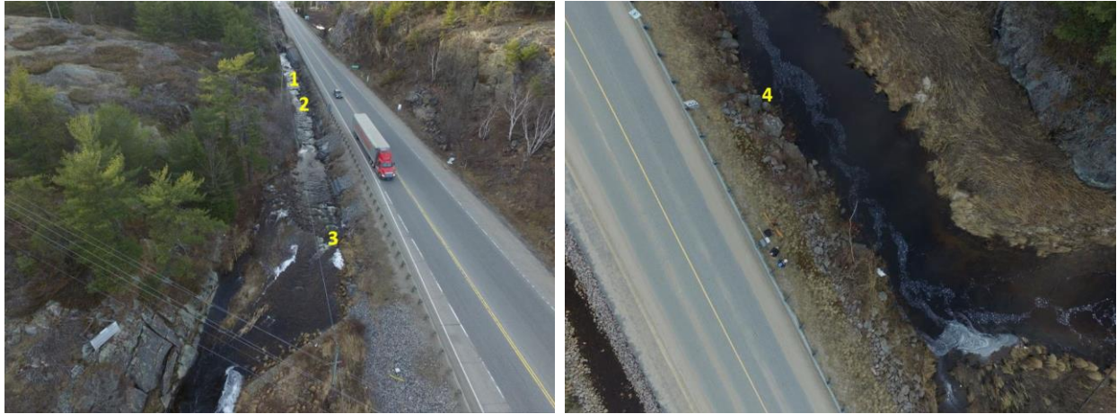
Figure 6. Water velocity (1-4) and water level stations (1,2,4) at the Sucker Creek spawning bed
