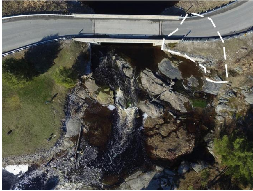
Figure 5. Dashed white line indicates the area of Dillon Rapids filled in from road development
