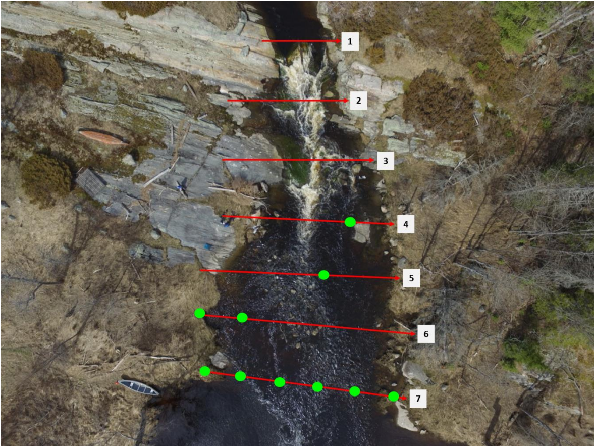
Figure 28. Spawning bed measurement transects at Young's Rapids. Green dots indicate ideal depth and substrate for Walleye spawning.
