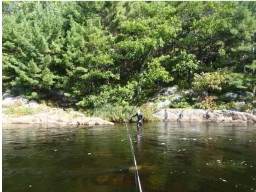
Figure 18. Measuring bankfull width and depths along transect 3
