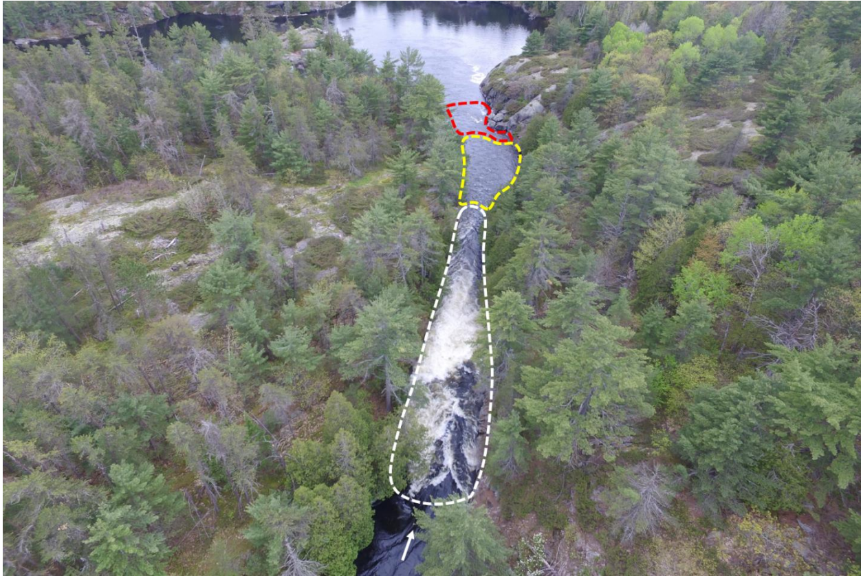
Figure 35. Spawning bed at Trestle Gully. Dashed white line indicates area of primarily bedrock and large boulder substrate. Dashed yellow line shows an area of primarily cobble and small boulders. Red dashed line highlights an area of primarily small and large boulders.
