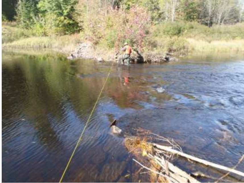
Figure 25. Measuring bankfull width and depths along transect 1
