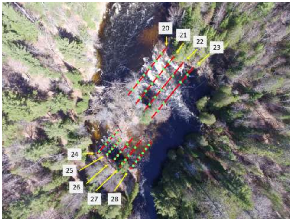
Figure 28. Spawning bed measurement transects 20-28 at the Harris Branch spawning bed. Green dots indicate points with ideal depth and at least some ideal substrate for Walleye, Lake Sturgeon, and/or Sucker spawning.
