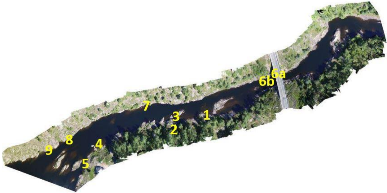
Figure 8. Water velocity (1, 3-6b, 7-9) and depth stations (1, 2, 4, 6a, 7-9) at Deadman's Rapids
