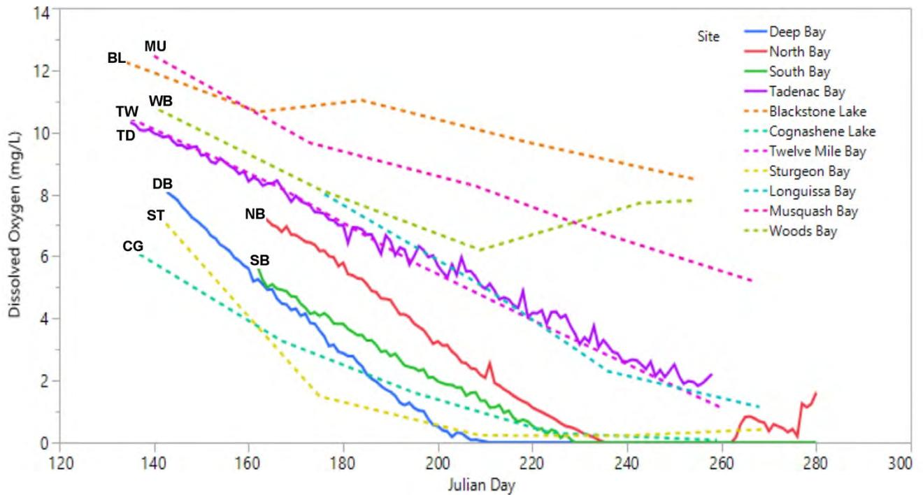
**Figure 3:** Changes in hypolimnetic dissolved oxygen (DO; mg/L) concentrations within each embayment at the deep station. Unbroken lines are for data collected with in-situ Onset HOBO U26-001 DO data loggers whereas dashed lines are for those collected at monthly intervals taken approximately 2 m above the sediment surface.
