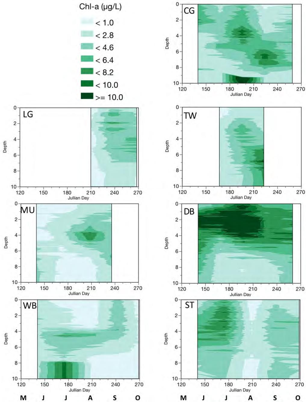
**Figure 13:** Chlorophyll-a (CHL-a) isopleths for six bays in this study. Data were obtained with a Turners C3 *in situ* submersible fluorometer. Corresponding data for Tadenac Bay, North Bay or South Bay are available from Environment Canada.
